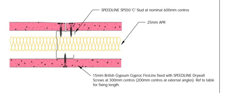
All performance data and system specifications are for systems constructed with materials & components as shown. The inclusion or substitution of any other manufacturers materials or components could invalidate test data and system performance and permission must be given in writing by SiG PLC.
